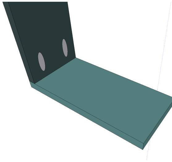
Next, measure 5 inches from the inside edge and mark on the small board. Attach next shelf piece here. See image below:
