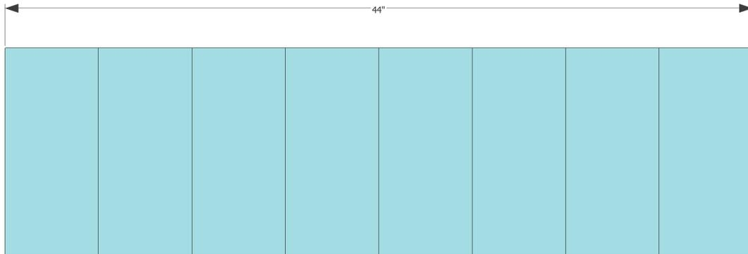
This will be the backboard of the shelf. Measure the width of these boards. That is the width of the shelf. You can adjust this as needed by adding or subtracting boards, ripping them, etc.
