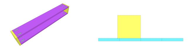
Use a Kreg clamp to hold each end piece to the long shelf board as you drive the screws.
